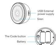
Notice: Pleases use USB power supply, the backup battery can only work for two days.Plug in the USB power supply and load the battery at the same time, then the sensor will work in priority.
